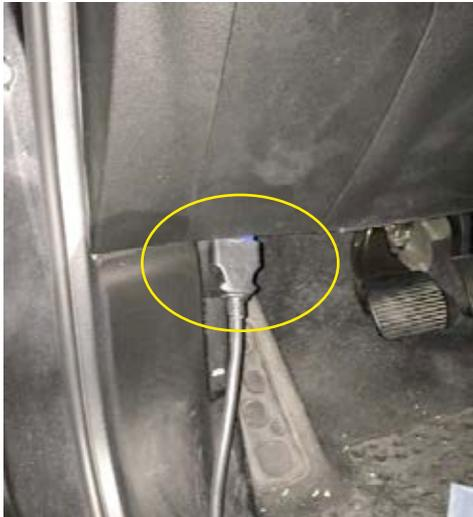
Port locations vary on different makes & models but are typically just under the dash on the drivers side and not too hard to find.
