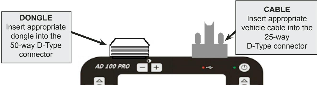
1) Connect the appropriate Dongle and diagnostic cable for the vehicle being programmed.
