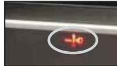
When the vehicle is started the theft light / indicator should be out. (Not blinking etc)
