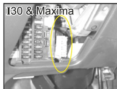
The 1999 Infiniti I30 & Nissan Maxima have a port located in the Fuse Panel.
