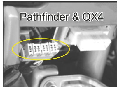
The 1999-2000 Infiniti QX4 & Nissan Pathfinder have the port exposed on the very bottom of the dash.
