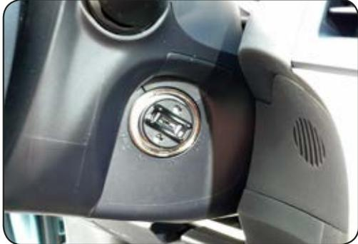
Insert the factory Emergency Key into the ignition lock cylinder and turn to the "Run" position.
