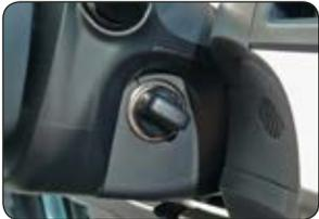
Next place the Prox Remote onto the Emergency key sticking out of the ignition.
