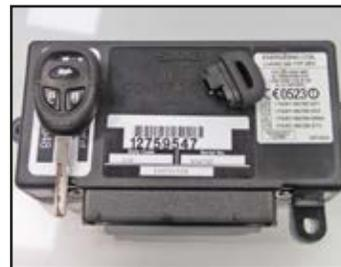
You need to have a working key to ADD more keys using the PRO. If no keys are available you must either REPLACE or Re-FLASH the TWICE module.
