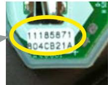
> The ID code is found on a white sticker attached to the circuit board on the inside of the remote. Open each remote you want to program and write down this ID before starting out. If the sticker is not there or cannot be read it you will not be able to proceed. The ID code is the top line on the sticker (8 digits & no letters).
