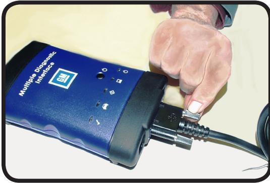
1. Connect the 26-pin end of the DLC cable to the bottom of the MDI, then tighten the screws.
